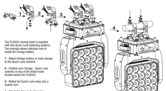
**4** - Attach the Omega fixations to a structure and lock them.
