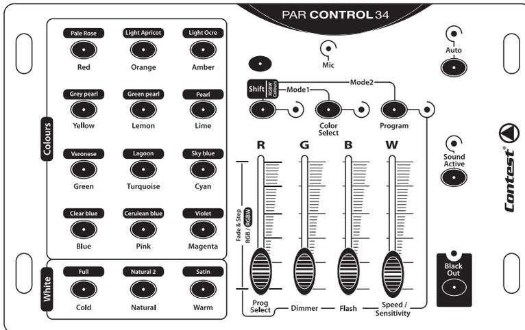
Your compatible projector must be assigned in DMX mode, its address must be 1 to be controlled via the PARCONTROL34.
